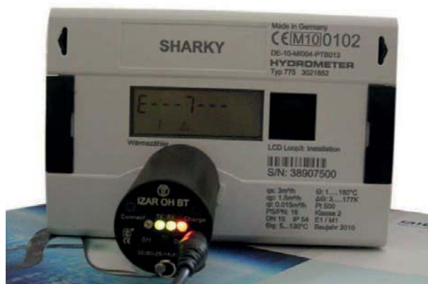
Fig. 4 Opto head on system device and switched on
