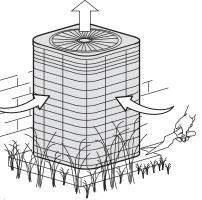
to work harder and use more energy. Keep shrubbery trimmed away from the unit and periodically check for debris which may have collected around the unit.
